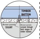
**CONTINUE PANELLING: Continue** panelling around the room fixing each panel to the battens with shower-panel adhesive, and/or screws through the back lip of grooved edge. Seal tongue and groove joints using shower-panel sealant.
