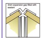
**BEGIN PANELLING:** First fix a internal corner profile in position ensuring that it is plumb. Apply shower-panel sealant to the recess of the profile. Apply shower-panel adhesive to the battens. Insert the first panel after removing the smaller tongue, or cutting to size. Then continue to panel away from the
