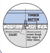
Vertical edges tongued and grooved giving finished panelling a smooth, easily maintained surface. Each panel has symmetrical tongued and grooved vertical edges to give 5mm of joint overlap. When sealed with Shower-panel sealant a waterproof joint is assured.
