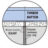
First trim off the tongues on the sides of each panel. Panels are easily cut on-site. The edges being covered by Shower-panel extrusions. This will facilate for faster installation. Panels can be joined together in continuous runs with decorative H joint extrusions.
